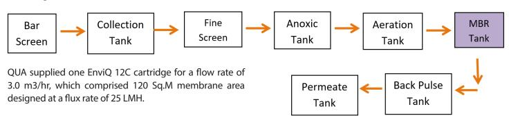
The MBR based STP was commissioned in February 2017. During commissioning, the Mixed Liquor Suspended Solids was steadily increased to 8000 mg/l, and has been maintained at the same level since then. The excess sludge is taken through the sludge handling system comprising sludge drying bed.
