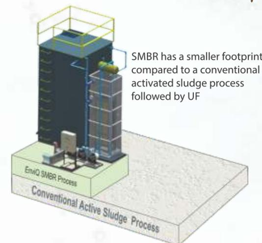
SMBR has a smaller footprint compared to a conventional activated sludge process followed by UF
