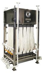
MBR combines conventional activated sludge technology with membrane filtration. MBR can be designed at a much higher mixed liquor suspended solids (MLSS) concentration compared to conventional processes, giving advantages of lower hydraulic retention time (HRT) and higher sludge retention time (SRT). In addition, MBR replaces clarifier/sedimentation tanks as well as media filtration. This reduces the footprint of the overall wastewater treatment.
